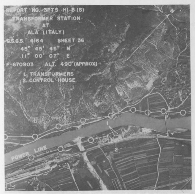
c. The transformer station at ALA (F-670903), at an approximate elevation of 490 feet, consisted of a single-storey building 60 feet by 300 feet and a two-storey building 30 feet by 80 feet. The transformer and switching bank were located just to the east of the building. There was a wall on the west side, approximately 50 feet from the transformer, which was not, however, a blast wall, and offered no protection. There were no known flak defenses of this installation.
