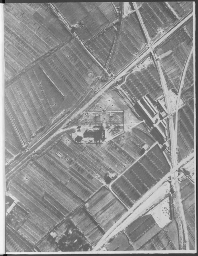
b. DOWEGLIARA: three bomb hits in the south end of the transformer yard destroyed two transformers, probably with slight damage to the two high-line towers immediately west of this point. At least three near misses were scored on the generator house, causing some damage. It was possible that the low wing of this building sustained a direct hit.
