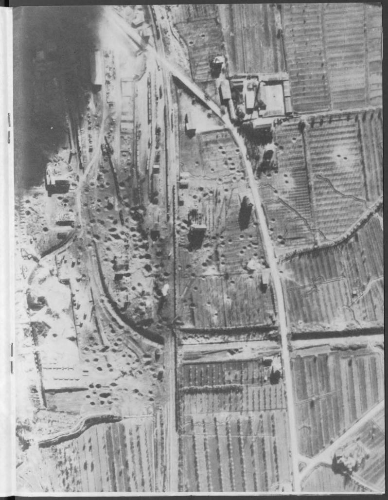
c. ALA: an extremely heavy concentration of hits was seen in the target area and in the area just to the east. The control house was very heavily damaged, the roof gone, and some of the walls badly ruined. No signs of fire could be seen. The transformer yard received at least six direct hits; the transformers themselves could no longer be seen, and it was assumed they had been destroyed.
